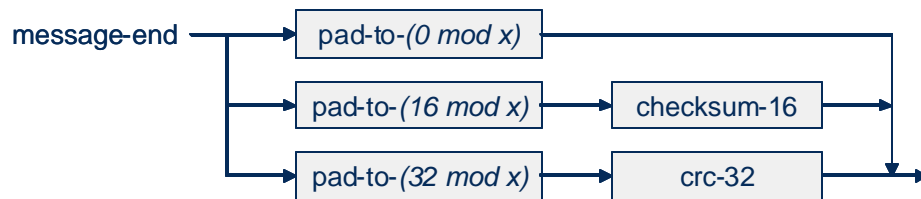
Figure 25 The syntax graph for message-end (x is the conveyance granule in bits)
