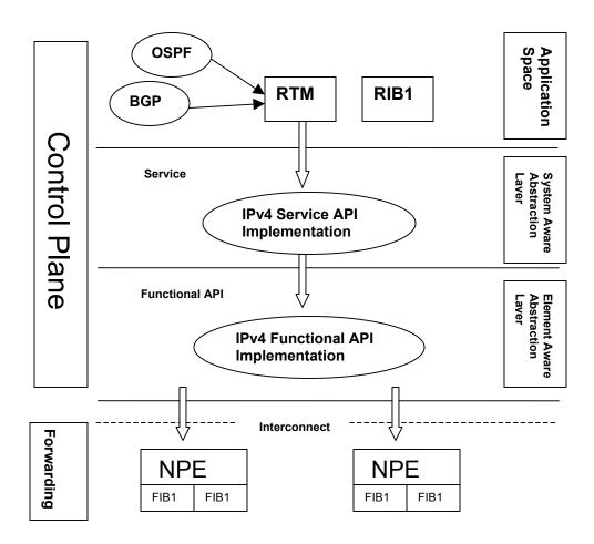
Figure 1 - Example Single FIB System
