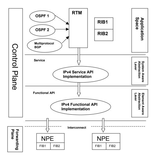
Figure 2 - Example Multiple FIB System
