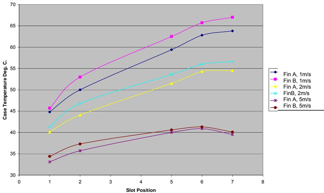
**Figure 14: Performance of Different Heat Sink Fin Geometry**
