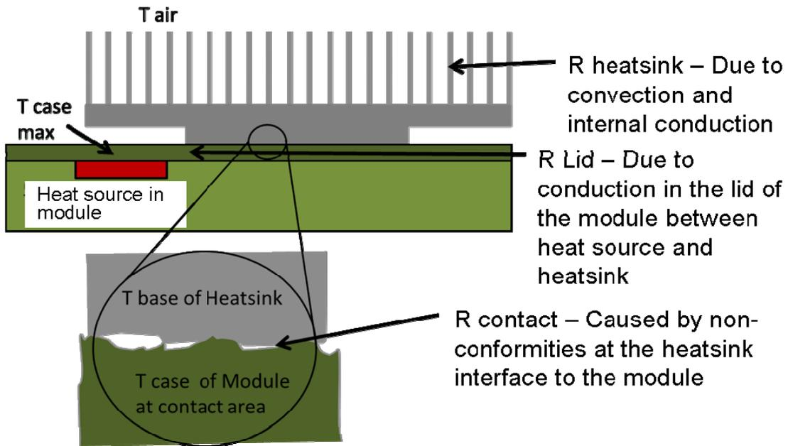
**Figure 13: Module to Host Thermal Interface**
