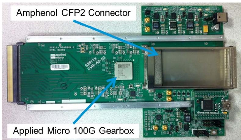
**Figure 9: Applied Micro CFP2 Evaluation Board**
