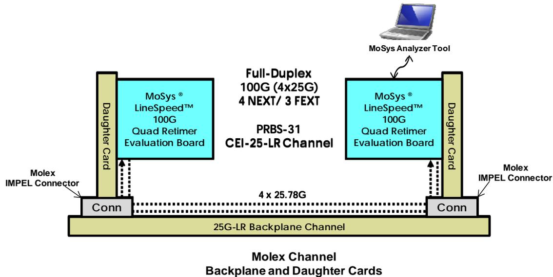
**Figure 17: Demo 8 Block Diagram**
