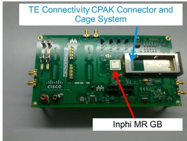
**Figure 6: Cisco / Inphi Evaluation Board**
