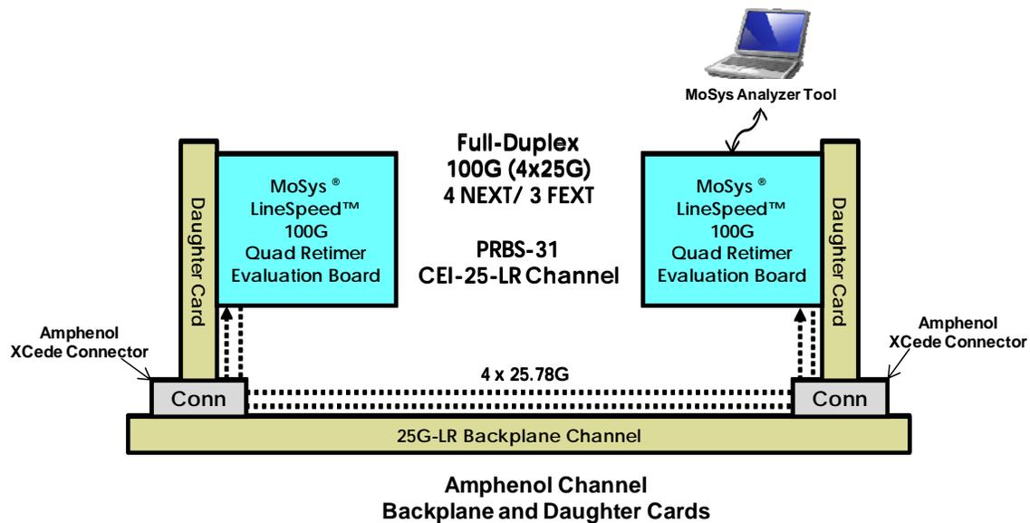
**Figure 16: Demo 7 Block Diagram**
