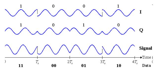
Figure 3. Independent modulation in-phase and quadrature signals which are added together to form a transmitted signal with QPSK modulation
