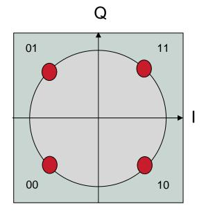
Figure 2. Representation of the association between signal phases and two bit data sequences.
