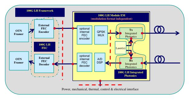
Figure 7. Block diagram of a transceiver module
