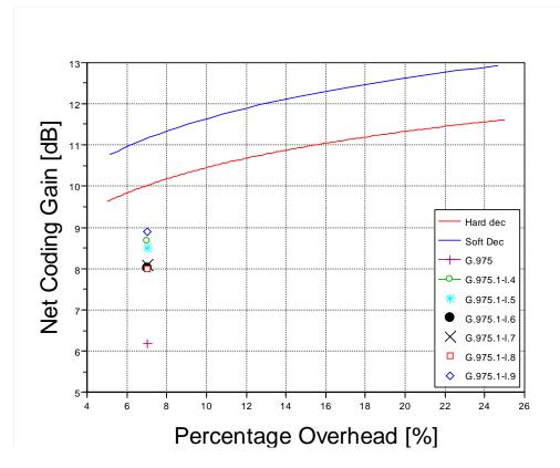
Figure 6. Theoretical limits and experimental results for performance achieved with several forward error correction codes.
