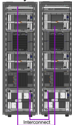
Figure 12 Rack to Rack side-by-side Interconnect Application Space
