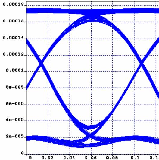
**Figure 6.1.2.1-3 NRZ-RB Transmitter Detected with a Rx with a BW at 60% the Bit Rate**
