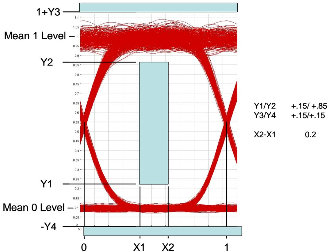
**Figure 6.1.1.1-1 Golden Transmitter Eye Mask**
