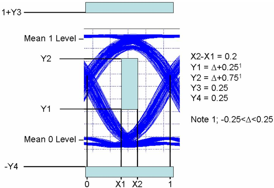
Figure 6.1.2.1-2 NRZ Amplified Eye mask with Realistic NRZ-RB Transmitter
