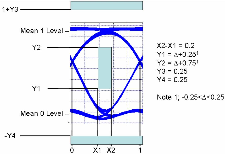
Figure 6.1.2.1-1 NRZ Amplified Eye Mask with Ideal NRZ-RB Transmitter
