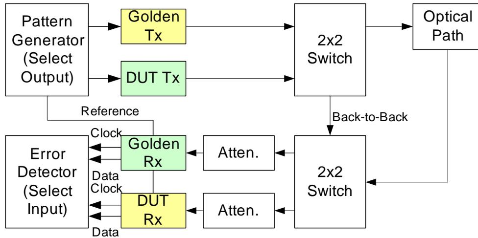
**Figure 7.3-1 Functional Block Diagram of a Notional Interoperability Test Set-Up Showing the DUT and the Golden Transmitter and Receiver**
