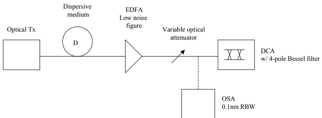
**Figure 9.1-1 Test Setup To Capture Eye Statistics**
