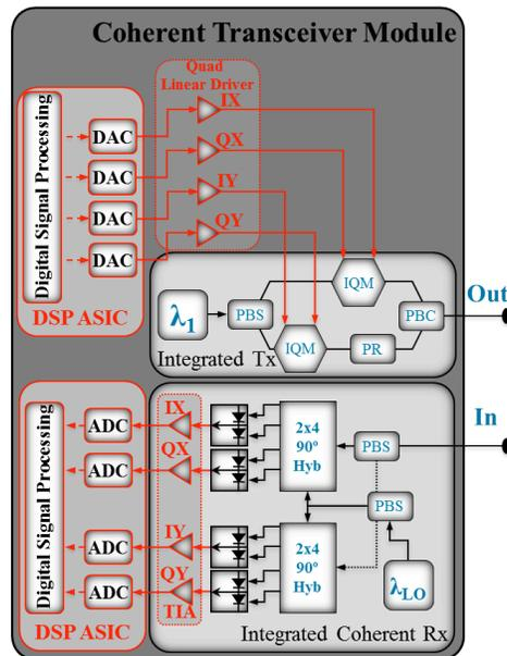
**Figure 2** Coherent transceiver concept design for PDM systems with an integrated transmitter and coherent receiver.  $\lambda$ : laser source; IQM: in-phase quadrature modulator; PBS: polarization beam splitter; PBC: polarization beam combiner; PR: Polarization Rotator; LO: local oscillator.
