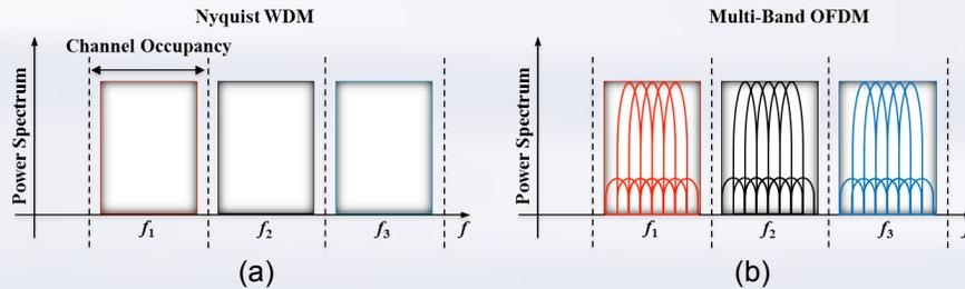
**Figure 6: Optical channel multiplexing for spectrally-efficient WDM networks. (a) Nyquist WDM. (b) Multi-Band OFDM.**
