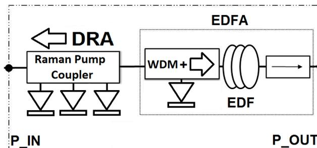
**Figure 9 Structure of a hybrid optical amplifier (three pumps DRA and single stage EDFA).**
