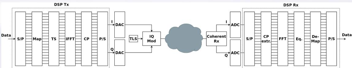
**Figure 8: Generic scheme for the generation and detection of OFDM signals. The DSP functions include serial/parallel (S/P) and parallel/serial (P/S) conversion, symbol mapping and demapping, cyclic prefix (CP) insertion and extraction, training sequence (TS) insertion, and equalization.**
