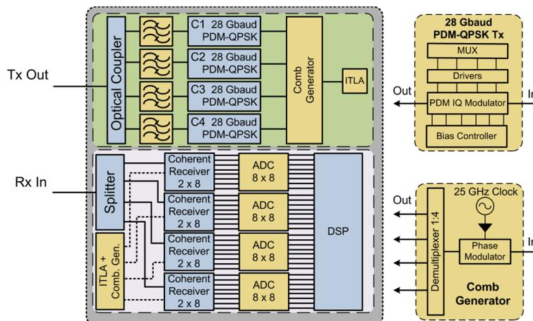
**Figure 15** Transceiver architecture for 400G long-haul applications based on 4x100G PDM-QPSK.
