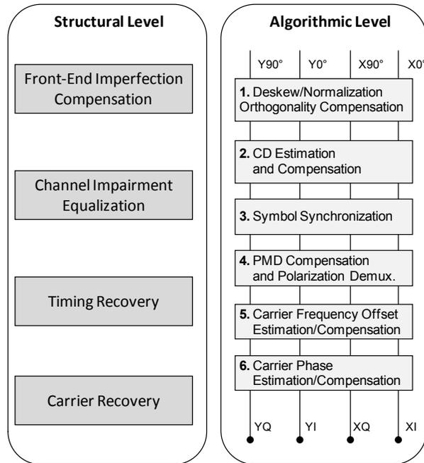
**Figure 4 DSP flow in a digital coherent optical receiver.**
