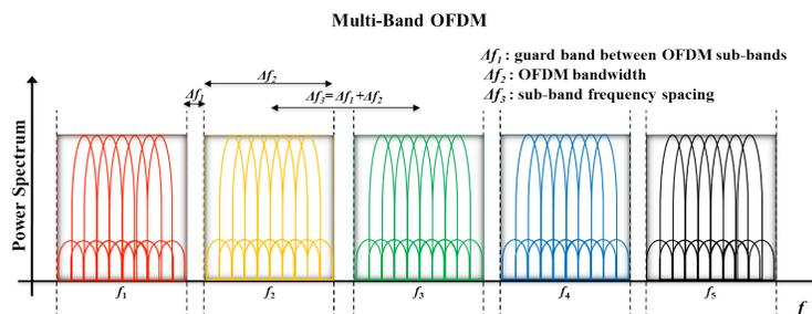
**Figure 13 Multi-band OFDM spectral allocation highlighting the guard band ( $\Delta f_1$ ), bandwidth ( $\Delta f_2$ ) and frequency spacing ( $\Delta f_3$ ) between the OFDM sub-bands.**
