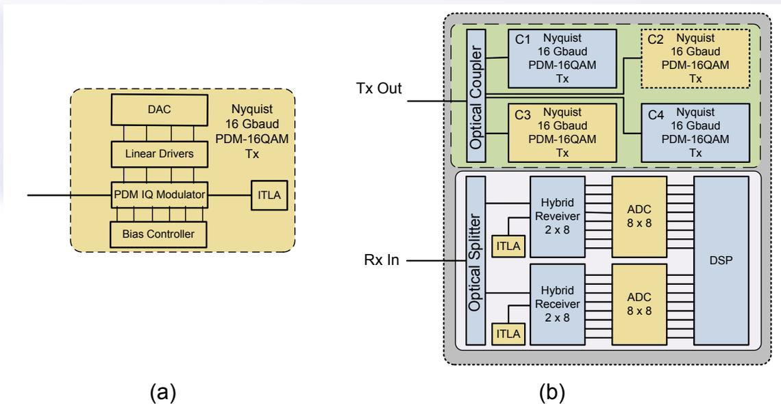
**Figure 16 Long-haul 400 Gb/s transceiver architecture. (a) One sub-channel transmitter block; (b) Transceiver complete module based on 4x100G PDM-16QAM.**
