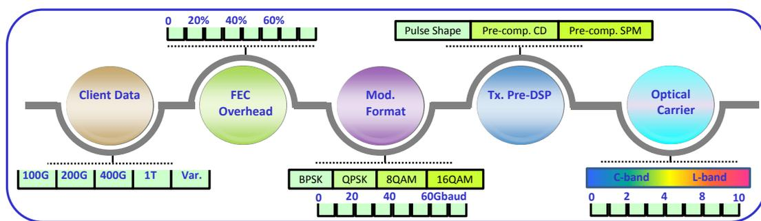
**Figure 11 Software defined optics for flexible 400G optical transceivers.**
