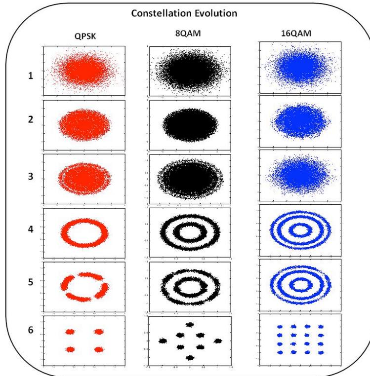
**Figure 5** Constellation evolutions for QPSK/8QAM/16QAM signals in a digital optical coherent receiver.
