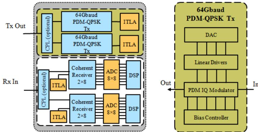
**Figure 14** Transceiver architecture for metropolitan application 2x200G PDM-QPSK.
