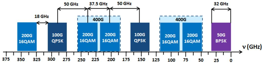
**Figure 1 New Flexgrid defined in ITU-T G.694.1 recommendation.**
