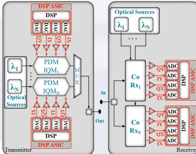
**Figure 7: Conceptual structure of a super-channel transceiver. CO Rx: Coherent Receiver; PDM-IQM: Polarization-Division Multiplexing IQ Modulator.**
