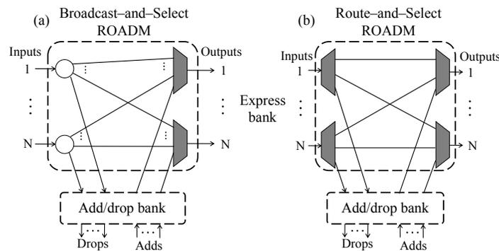
**Figure 10 (a) Broadcast-and-Select and (b) Route-and-Select ROADMs.**
