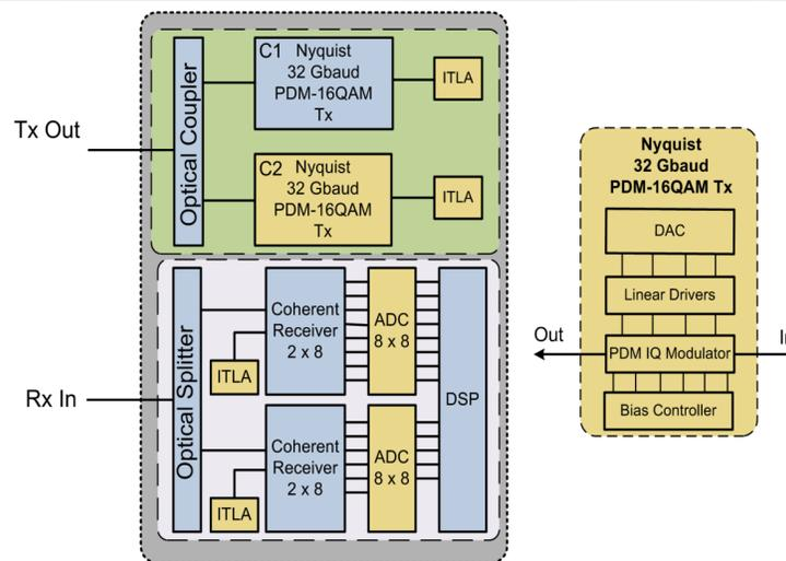
**Figure 12 Transceiver architecture for metropolitan application 2x200G PDM-16QAM.**
