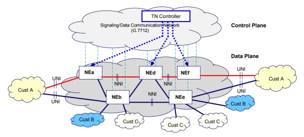
Figure 5: Concept #3 - Use SDN controller to control each network element individually
