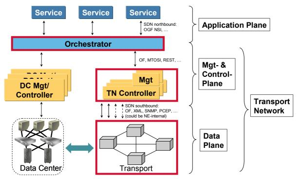
Figure 2: SDN reference architecture; the Transport SDN components covered by this document are marked red
