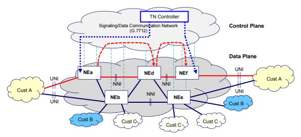
Figure 3: Concept #1 - Use SDN to provision packet mapping into optical paths
