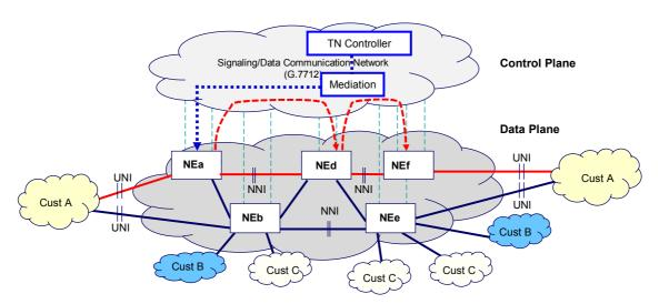
Figure 4: Concept #2 - Use SDN as a programmatic interface to the service provider network
