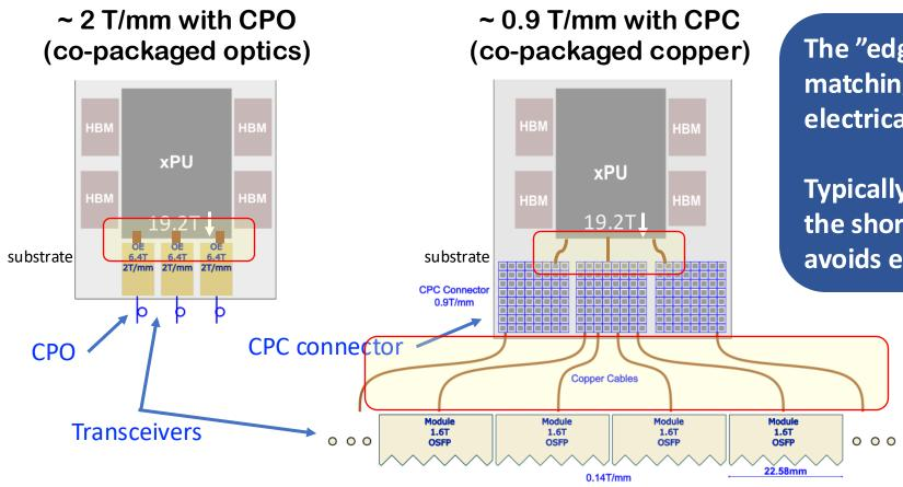
The "edge density" requirement comes from matching the transceiver density to the electrical interface density at the ASIC
