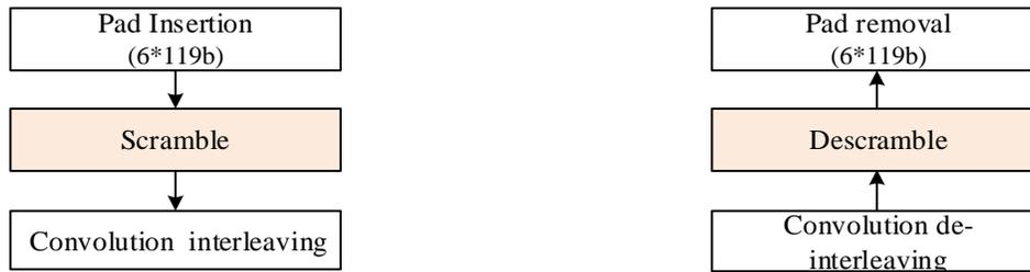
**Figure 29: Frame synchronous scrambler**
