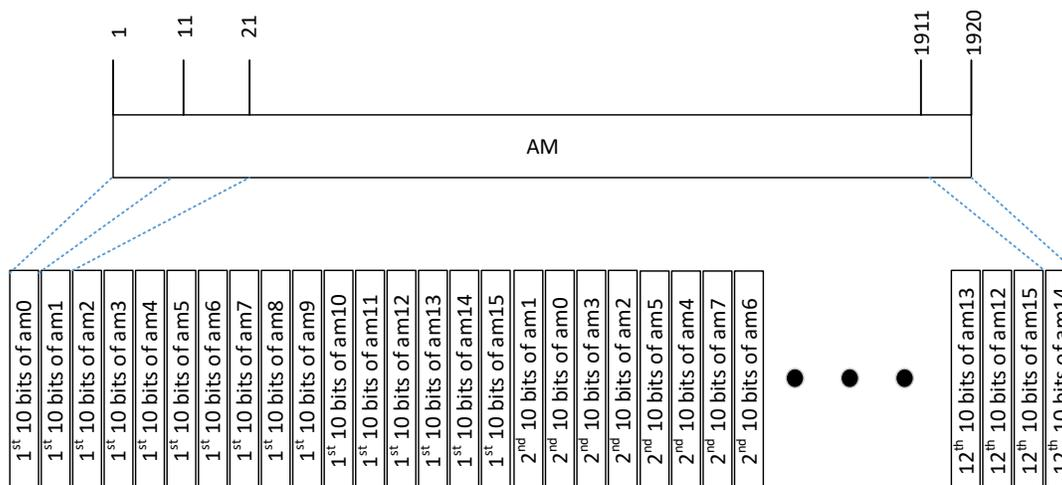
**Figure 11: Alignment Marker transmission order – 10b interleaved**
