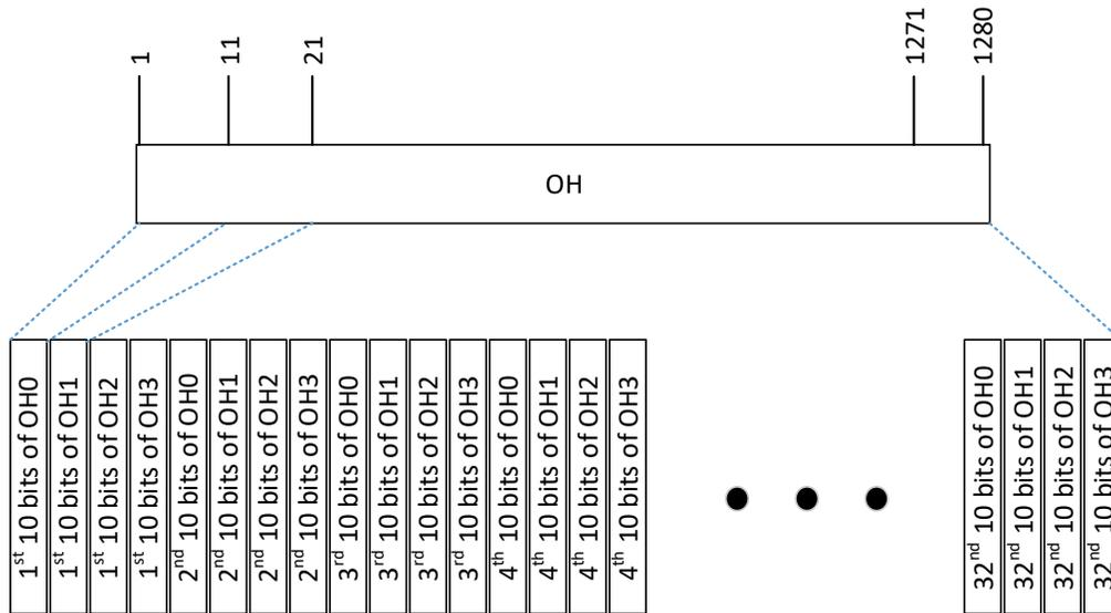
**Figure 14: Over Head transmission order – 10b interleaved**
