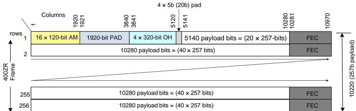
**Figure 10: 400ZR frame structure with parity bits**
