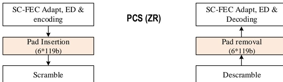
Figure 27: Pad insertion/removal
