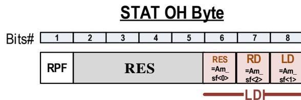
**Figure 18: STAT Over Head byte definitions**
