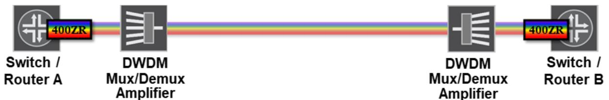
Figure 3: Switch/Router line card with 400ZR DWDM Interfaces
