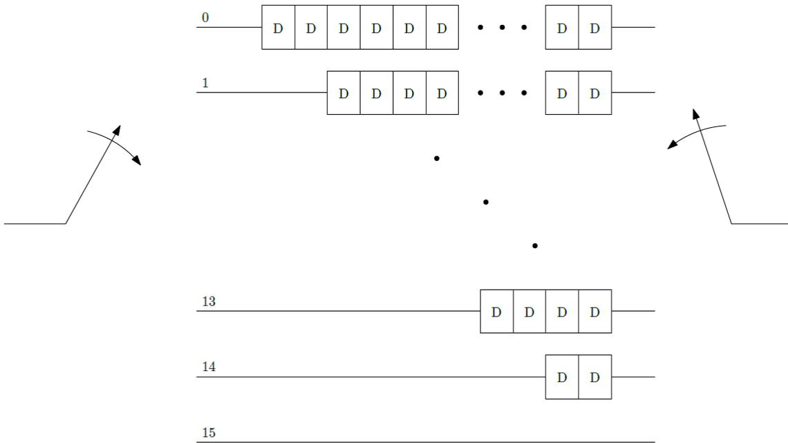
**Figure 31: Convolution interleave**
