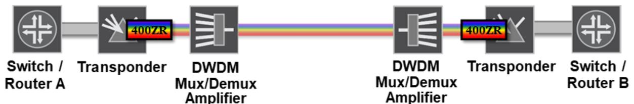
Figure 4: Transceiver line card with 400ZR DWDM interfaces
