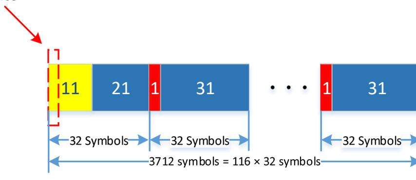
**Figure 36: DSP sub-frames 2-49 of the DSP super-frame**
