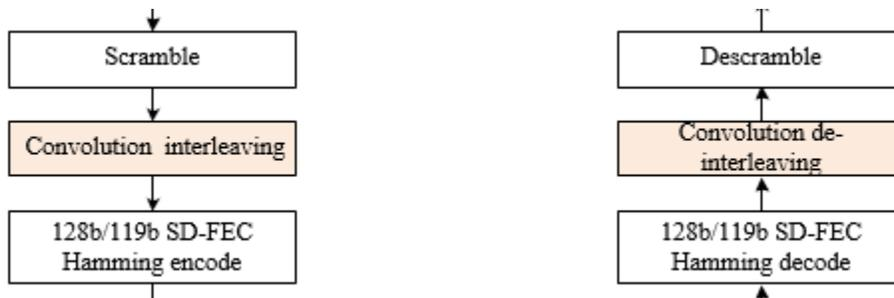
**Figure 30: Convolution interleave**
