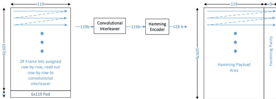
**Figure 32: Hamming FEC frame format**
