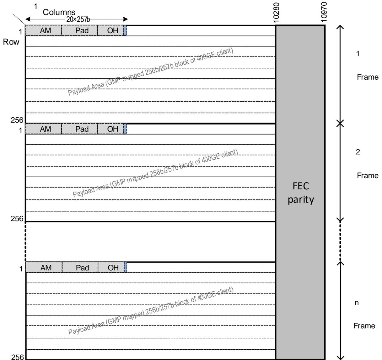
Figure 9: 400ZR multi-frame structure with parity bits
