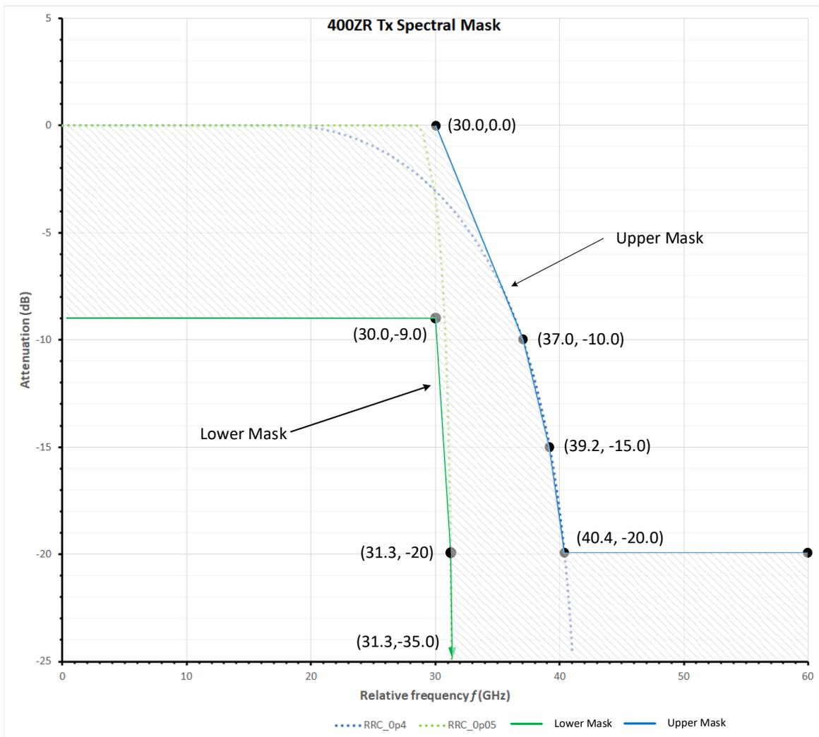
**Figure 43 Transmit Spectral Masks (Min and Max)**
