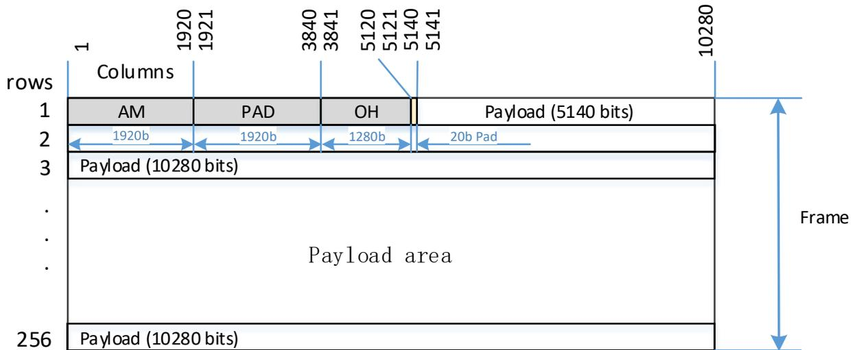
**Figure 8: 400ZR frame structure without parity bits**
