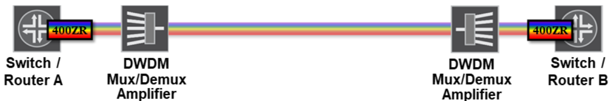
Figure 3: Switch/Router line card with 400ZR DWDM interfaces
