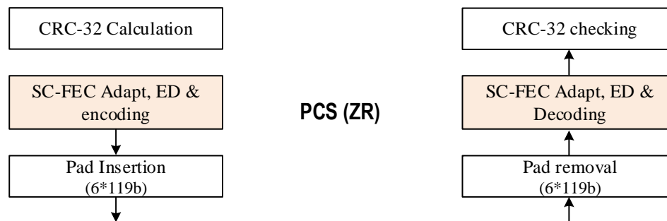
Figure 26: 400ZR HD-FEC processes
