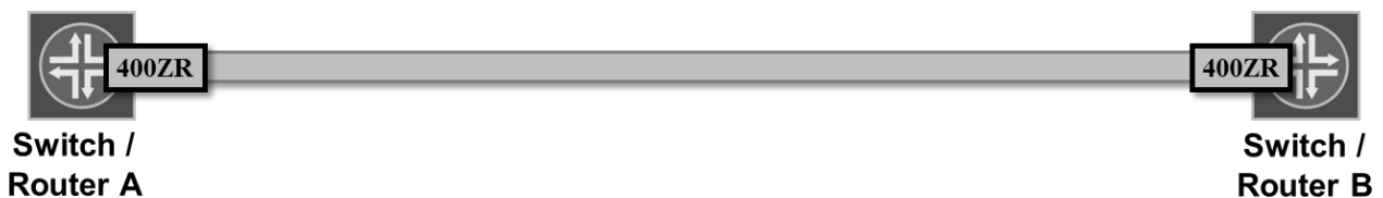
Figure 6: Router/Switch line card with 400ZR unamplified point-to-point interface
