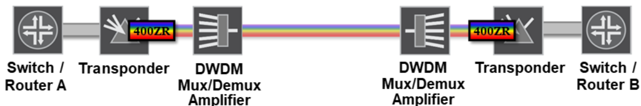
Figure 4: Transceiver line card with 400ZR DWDM interfaces
