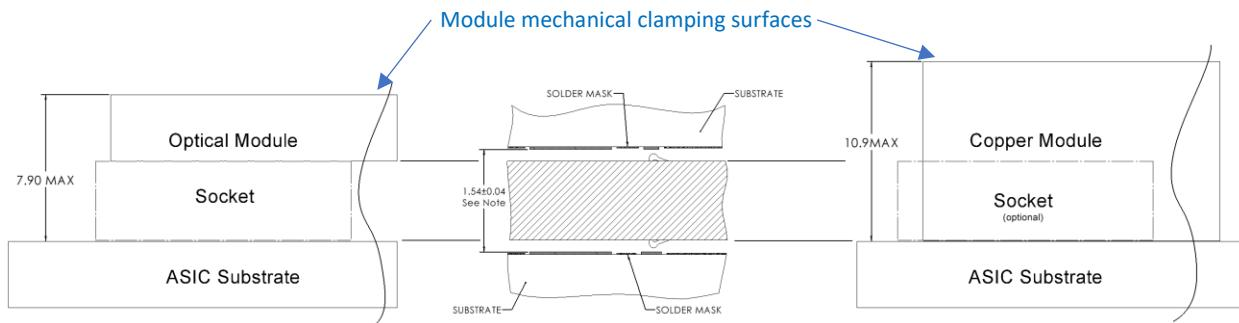
**Figure 18 Socket Height and Tolerance (see notes below)**
