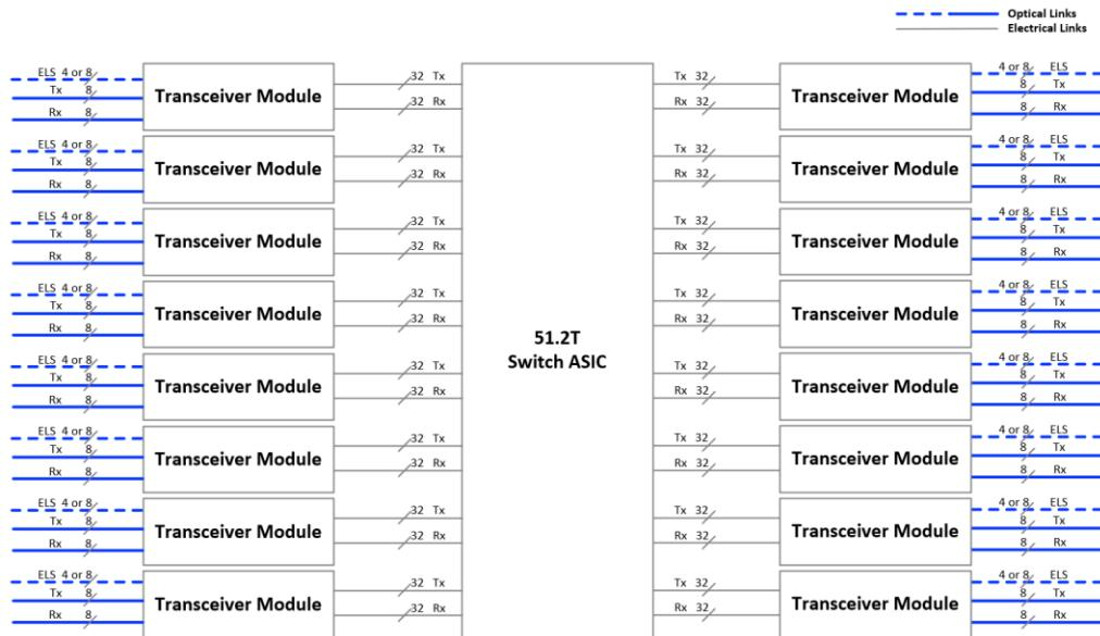
**Figure 2 High-level system block diagram (Optical)**
