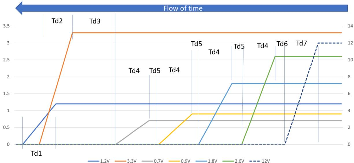
**Figure 8 Module Deactivation Supply Sequencing**
