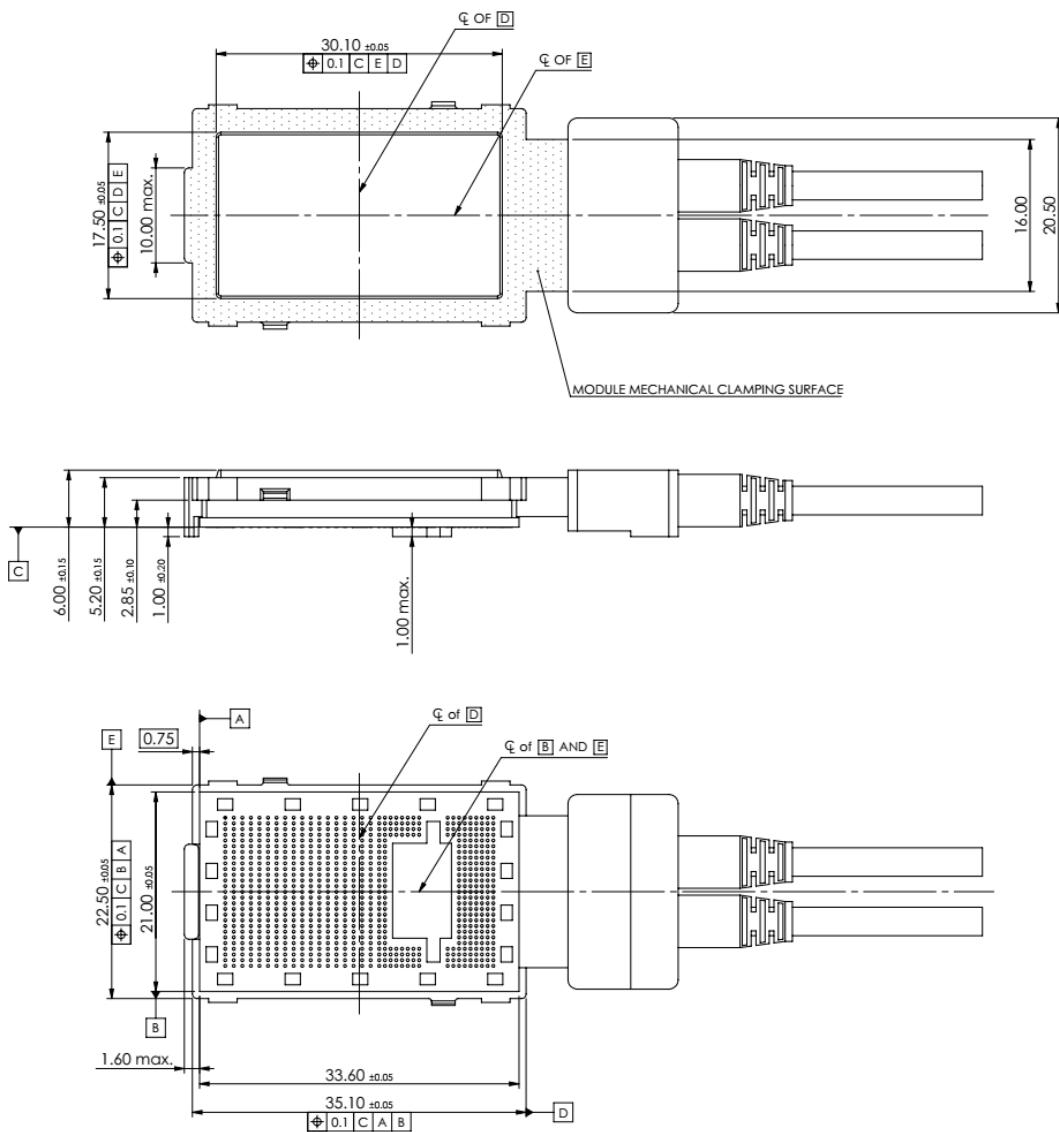
**Figure 12 Module mechanical dimensions**
