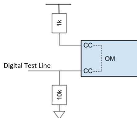
**Figure 11 Connectivity Check (CC) pin schematic**
