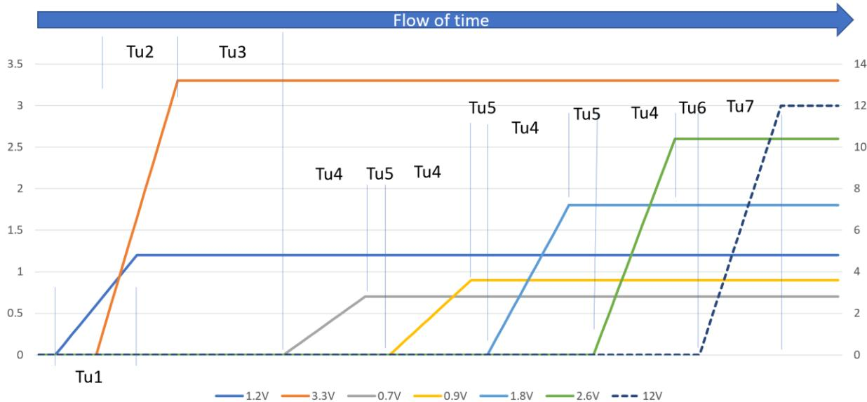
**Figure 7 Module Activation Supply Sequencing**
