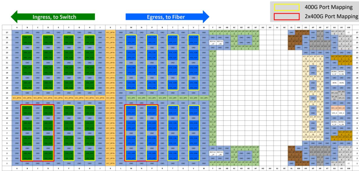
Figure 10 Electrical pins of 3.2 Tbs/s transceiver module (Top View)
