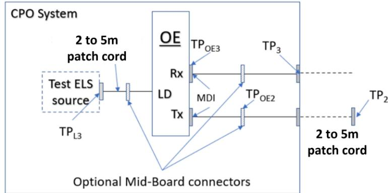
**Figure 9 Optical test points for the 3.2T Module**
