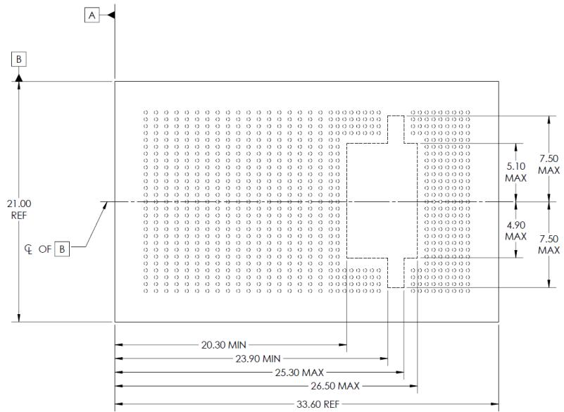
**Figure 15 Pad area keep out dimensions for module**
