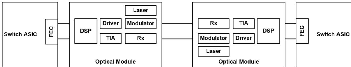
**Figure 6 Arrangement of FEC correction**
