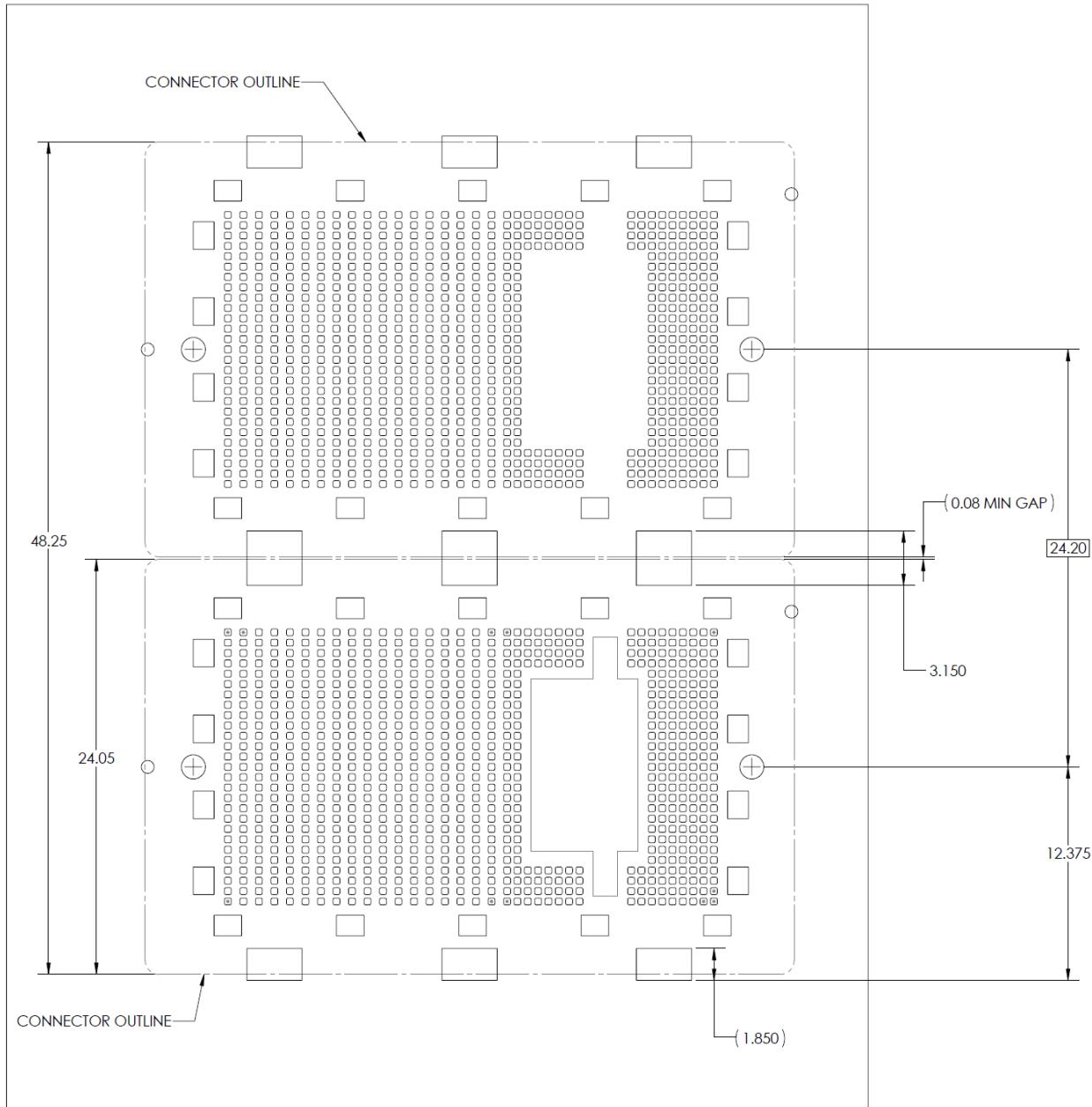
**Figure 17 Abutment of Module Socket Footprints**
