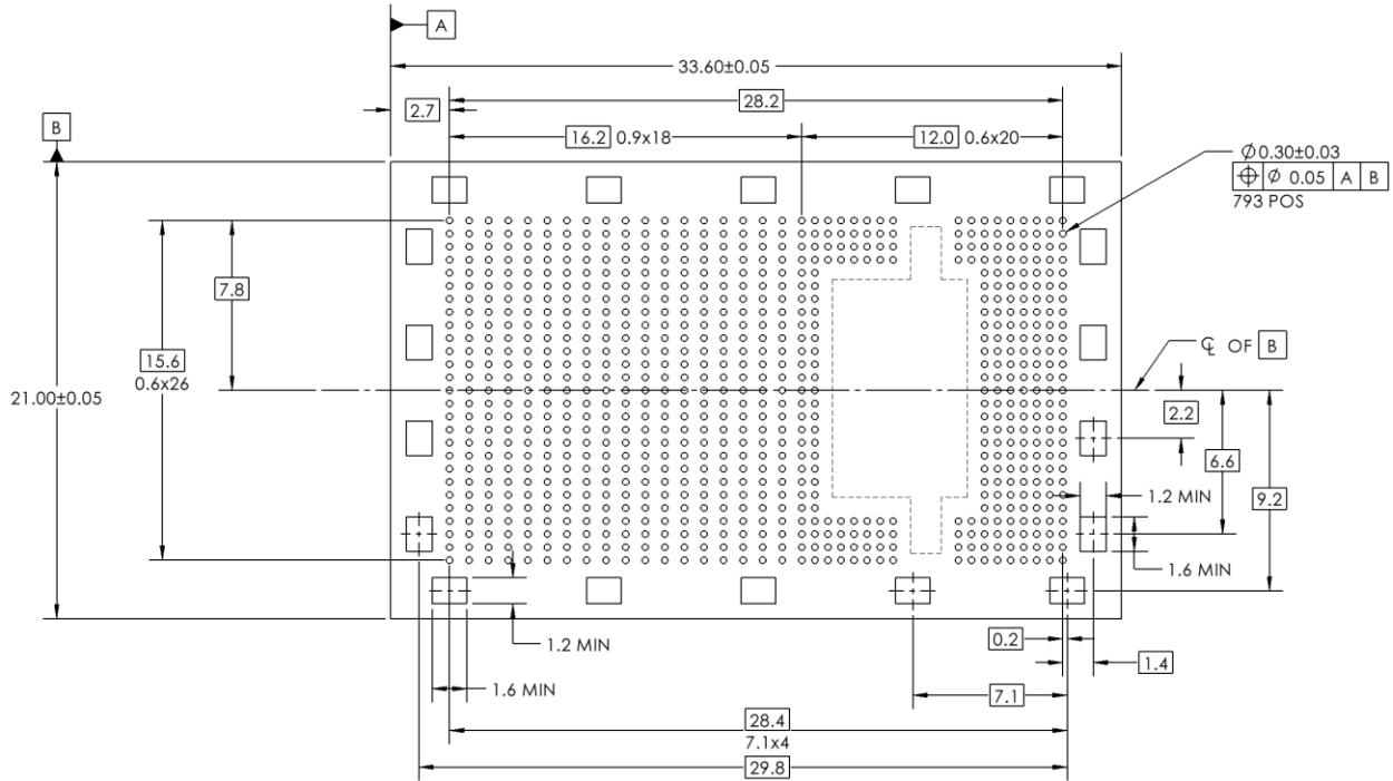
**Figure 14 Module mechanical footprint (see notes below)**
