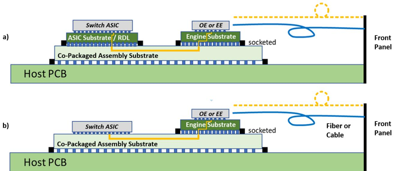
**Figure 5 Typical electrical channel implementation options: a) with ASIC package/substrate; b) without ASIC package/substrate**
