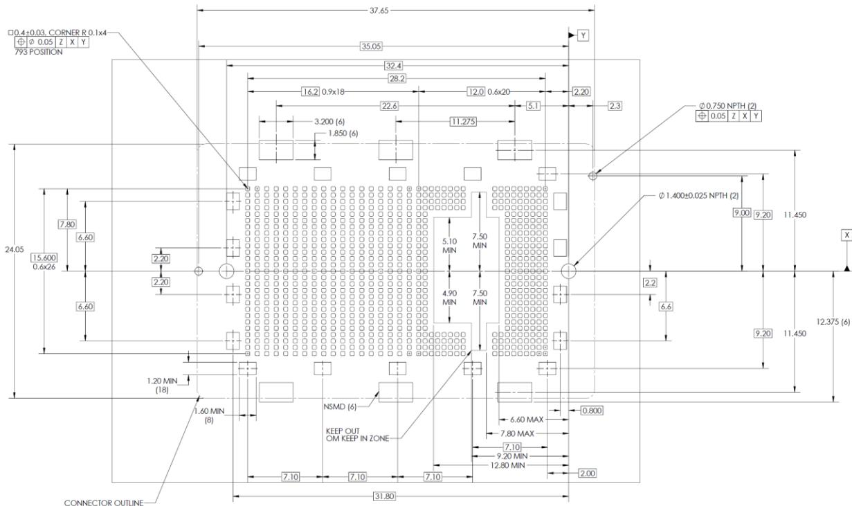
**Figure 16 Substrate socket mechanical footprint (see notes below)**
