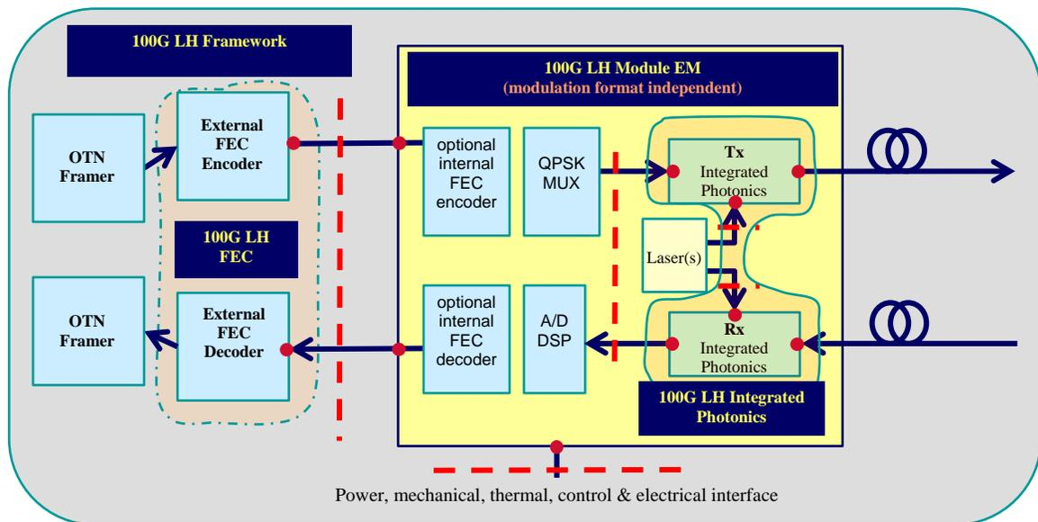
Figure 7. Block diagram of a transceiver module
