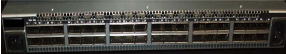
Figure 20 Pluggable Modules on Front Faceplate
