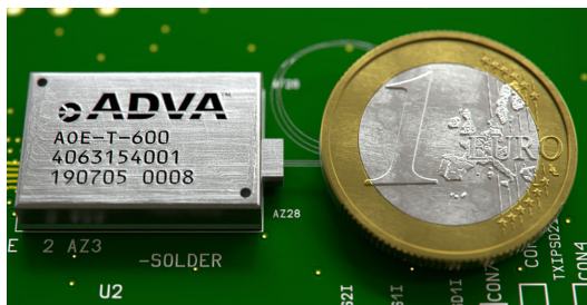
Figure 1: Type-1 Optical BGA IC-TROSA. 100-600Gb/s coherent modulator/driver/receiver in a single integrated SMT package.
