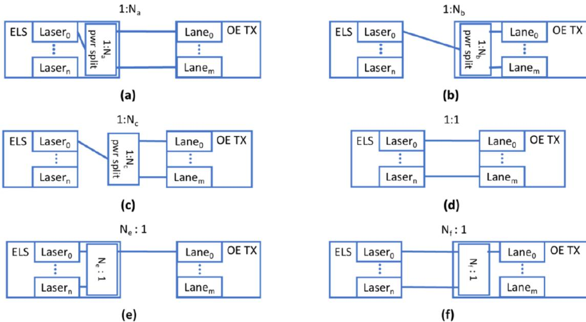
**Figure 4: Relationships for delivering optical power from ELS to OE**
