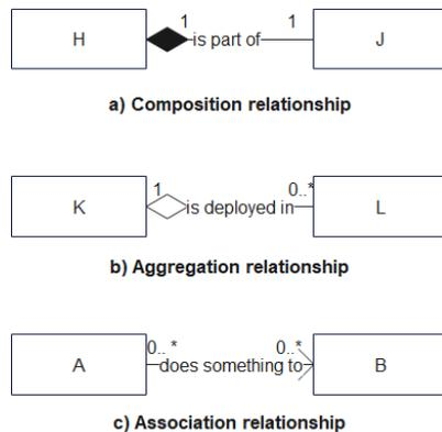
Figure 15 Legend for UML diagram used in this document
