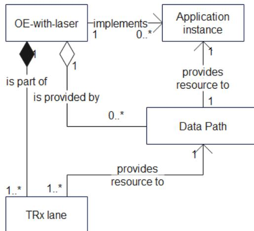
**Figure 10: Data Path, using optical engine with internal laser**
