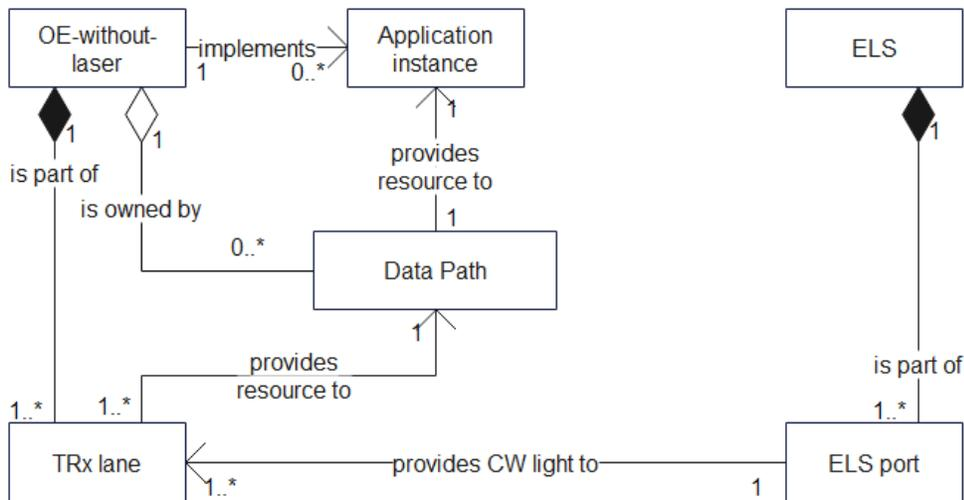
**Figure 12: Creation of a Data Path, using optical engine and external light source**
