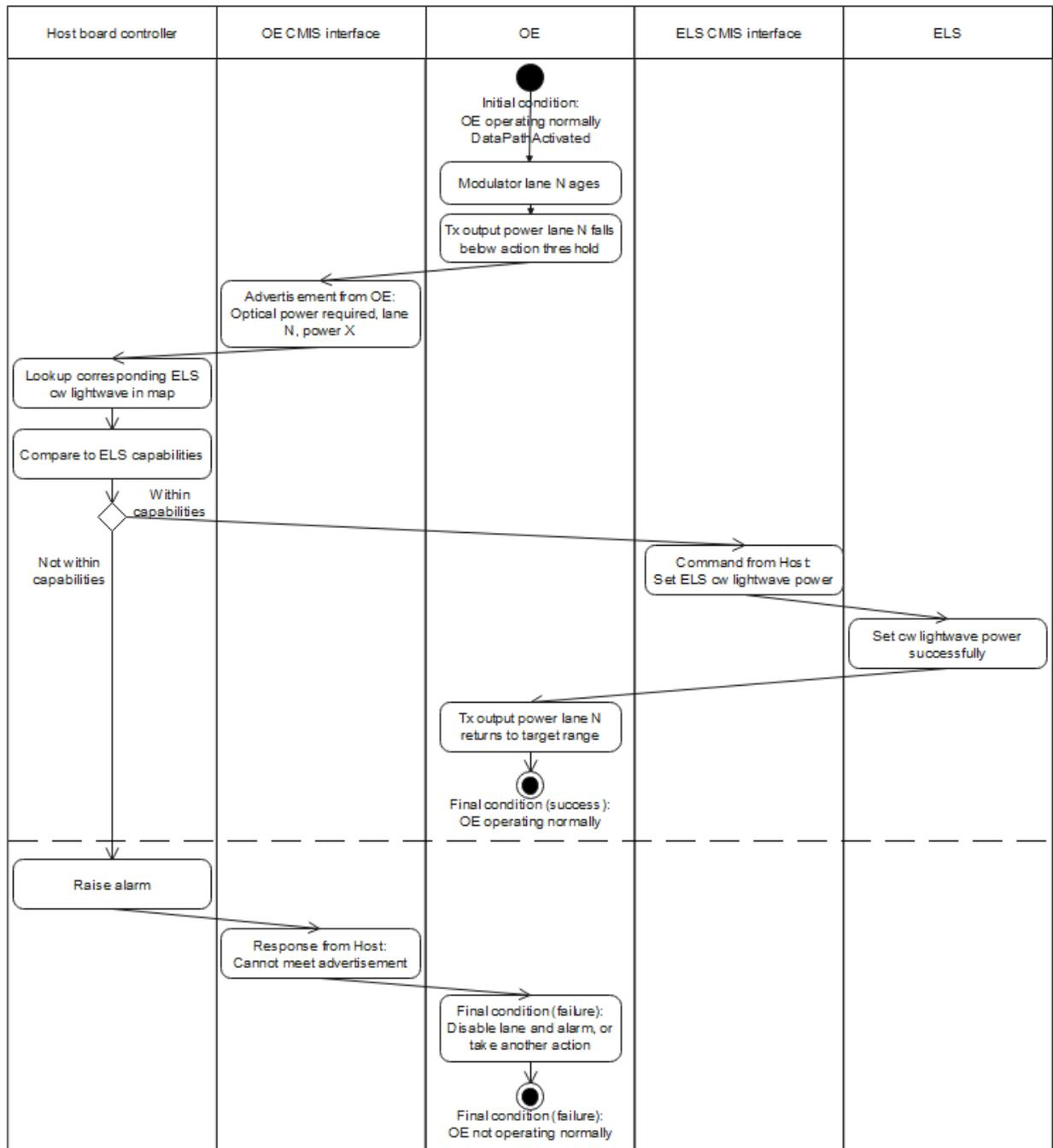
**Figure 13: Example use case: OE needs more CW light power due to OE aging**
