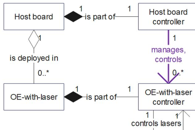
**Figure 3: Management architecture for Optical Engines with internal lasers**
