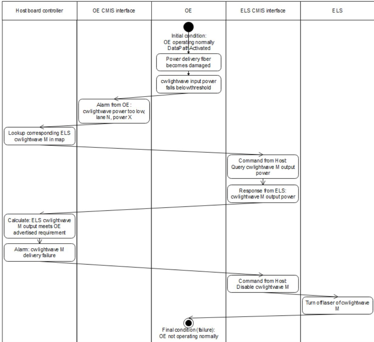
Figure 14: Example use case: Fault in power delivery fiber
