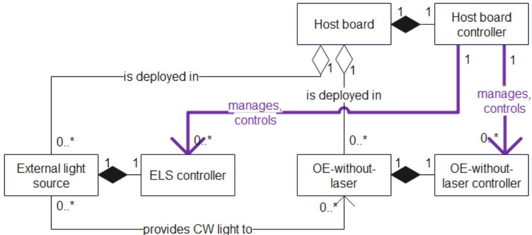
**Figure 8: Management architecture for Optical Engines with external light sources on host board**
