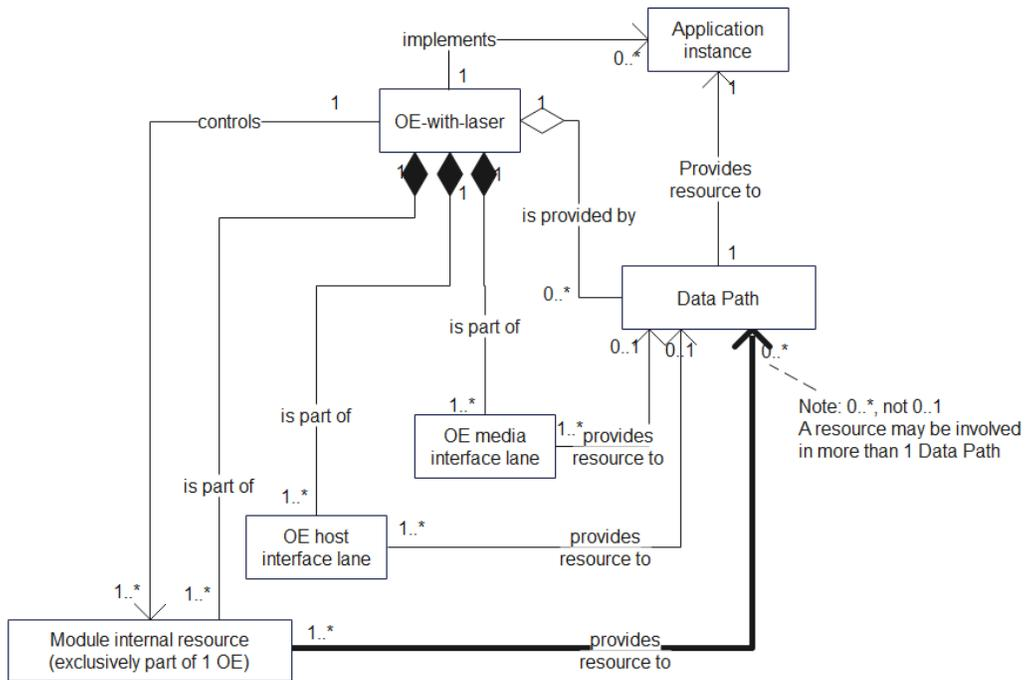
**Figure 11: Data Path, using optical engine with internal laser – detailed view**
