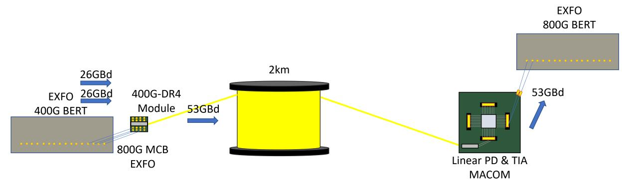
This interoperability demo consists of the linear conversion of an optical input from a 400G DR-4 module sent over 2km of SMF to an electrical signal via PD+TIA. The electrical signal is then sent through an OSFP connector to a BERT which integrates receive FFE functionality and achieves a link BER which exceeds standard requirements. There is no discrete DSP in the Rx path before the BERT, saving module power and cost.
