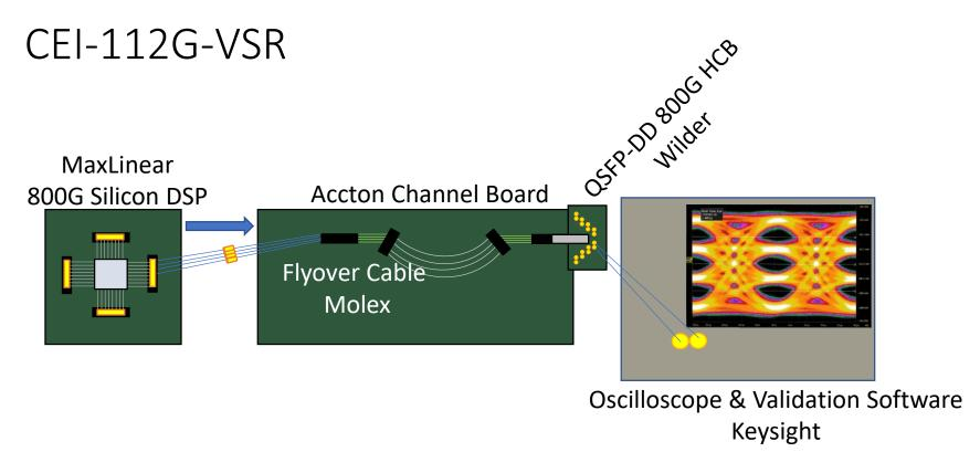
This demo uses a DSP/CDR to drive a channel loss emulating high density line card implementations, delivering an eye-opening exceeding target TP1a draft targets.
