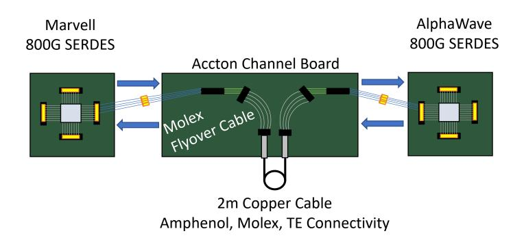
This interoperability demo consists of multivendor LR silicon transmitting 106.25 Gbps PRBS31Q PAM4 signals over a multivendor LR channel emulating high density 256x100G (25.6T) and 512x100G (51.2T) line card implementations while exceeding the BER target requirements.
