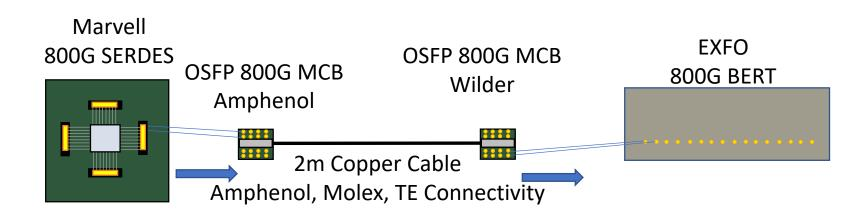
These interoperability demo's consists of multivendor LR silicon and silicon to test equipment transmitting 106.25 Gbps PRBS31Q PAM4 signals over a 2m Copper Cable and Module Compliance Boards while exceeding the BER target requirements.
