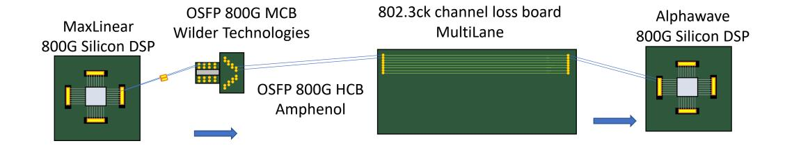
This interoperability demo consists of multivendor MR silicon transmitting 106.25 Gbps PRBS31Q PAM4 signals over a multivendor MR channel consisting of a mated compliance set of test fixtures and channel loss board at a bit error rate in of 1E-10.
