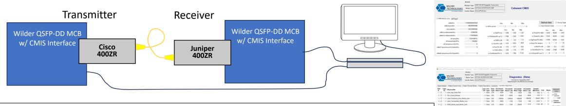
Laptop changes laser output power in transmitter via CMIS. Operation receiver EVM is reported back through CMIS VDM as well as other parameters reported through C-CMIS extensions.
