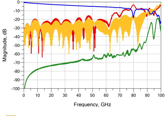
Insertion Loss Return Loss, Module side Return Loss, Host side PowerSum Crosstalk
